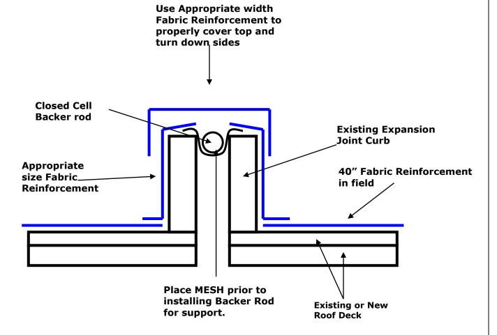
\* Overlap for Fabric Reinforcement is a minimum of 3" inches
